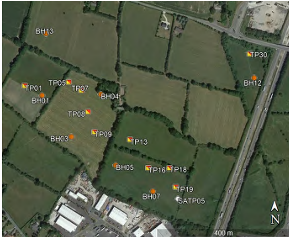
Figure 27 – Trial pits and boreholes where groundwater entry was recorded (initial 2022 phase of investigation)
