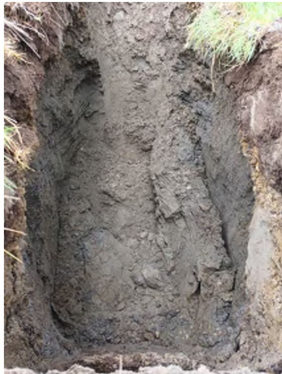
Figure 28 – Sidewall collapse in grey silty SAND upon completion of TP/RO09 excavation.
